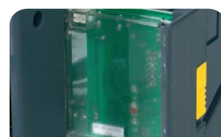
BOARD EASILY EXTRACTIBLE FROM THE OUTSIDE
